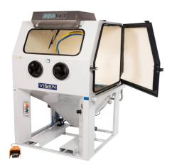
Sydney Vapour Blasting uses genuine Vixen Wet Blasting machinery to harmoniously recondition *Automotive, Motorcycle, Marine, Aeronautical* and other industrial components to the highest standard. The process uses a water and abrasive slurry to simultaneously blast and degrease which prevents impregnation of media onto the component.
